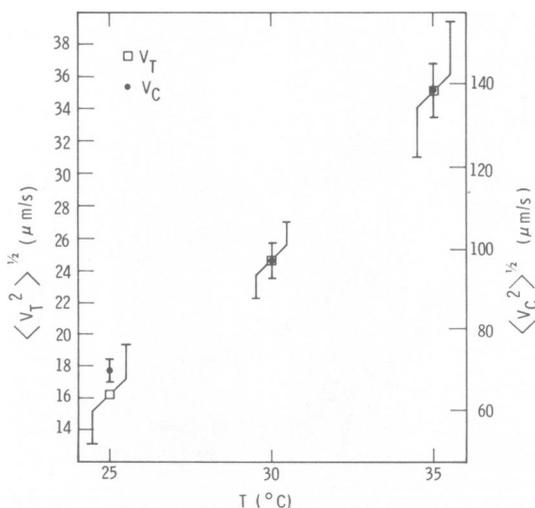
FIGURE 2 Temperature dependence of  $\langle V_T^2 \rangle^{1/2}$  and  $\langle V_C^2 \rangle^{1/2}$ . The error bars represent our estimate of confidence limits based on the repeatability of measurements at each temperature.
